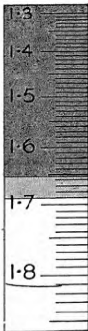
Figure 5. Shows, in a similar manner, the two edges which are seen with a peridot at their maximum possible separation 1.653-1.690
